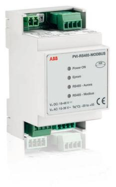
PVI-RS485-MODBUS is the ABB devices family able to convert the proprietary Aurora Protocol to ModBus RTU or ModBus TCP communication protocol.
