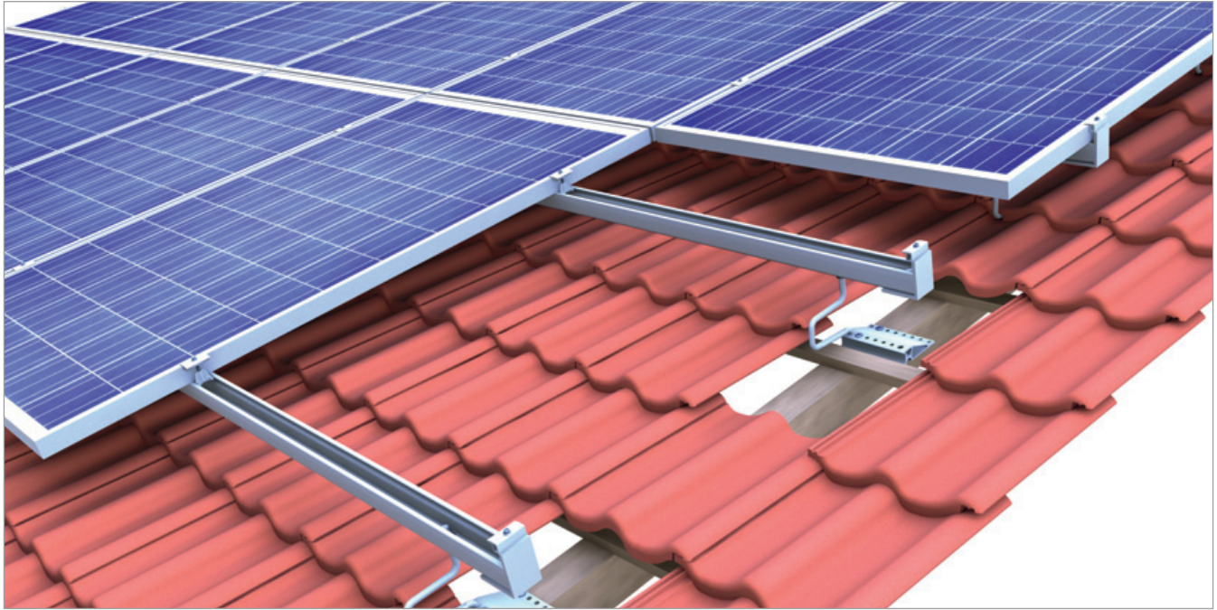
novotegra top-fix – single-rail clamping system with modules installed in portrait
