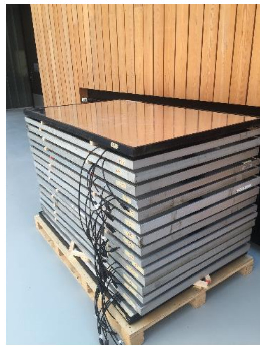
Figure 6: Some of the PV modules prepared with an aluminium foil
